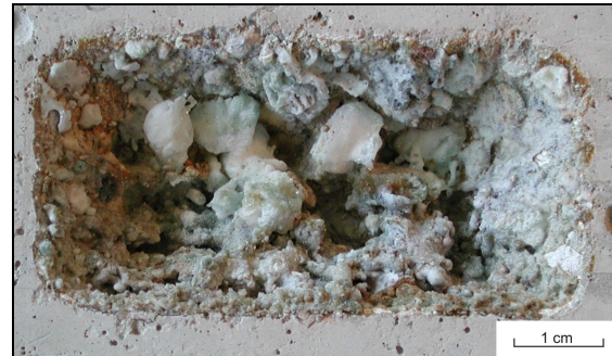
Fig.2: surface area of concrete after laser treatment
