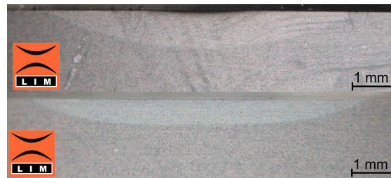
Fig. 3 Cross section view of laser hardening tracks in steel 1.2379: above: obtained by use of a conventional focusing optics; below: obtained with the specific optics (see text) that had been developed for laser hardening and cladding made with 80 % of laser power.
